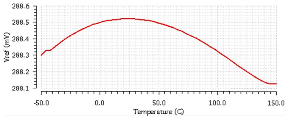
Fig. 4. Output voltage of the proposed Sub-1V CMOS reference voltage generator over the extended temperature range from  $-50^{\circ}\text{C}$  to  $150^{\circ}\text{C}$ , at the typical corner and with supply voltage of 1 V.
