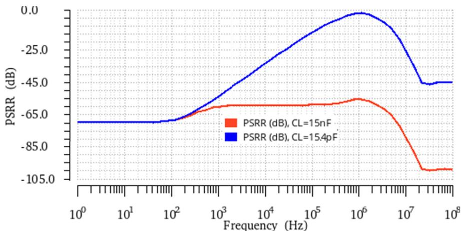
Fig. 10. PSRR of the output voltage for 1 V supply and at room temperature.
