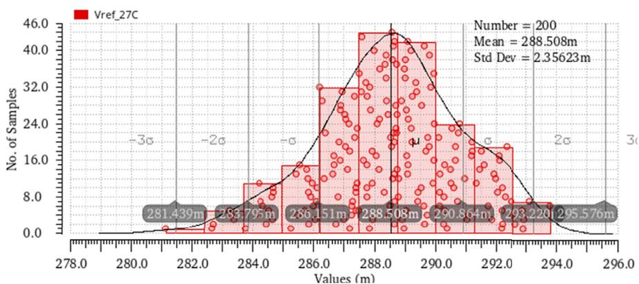
Fig. 12. Monte Carlo simulation results at 27 °C at the supply voltage of 1 V.
