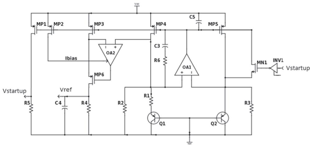
Fig. 1. The proposed sub-1V CMOS reference voltage generator.
