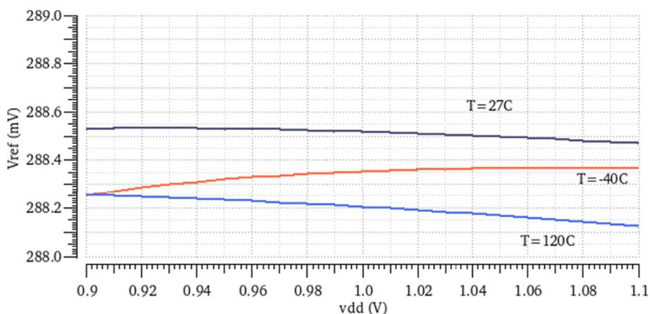
Fig. 11. Line sensitivity of the proposed voltage reference at 27 °C, -40 °C and 120 °C.
