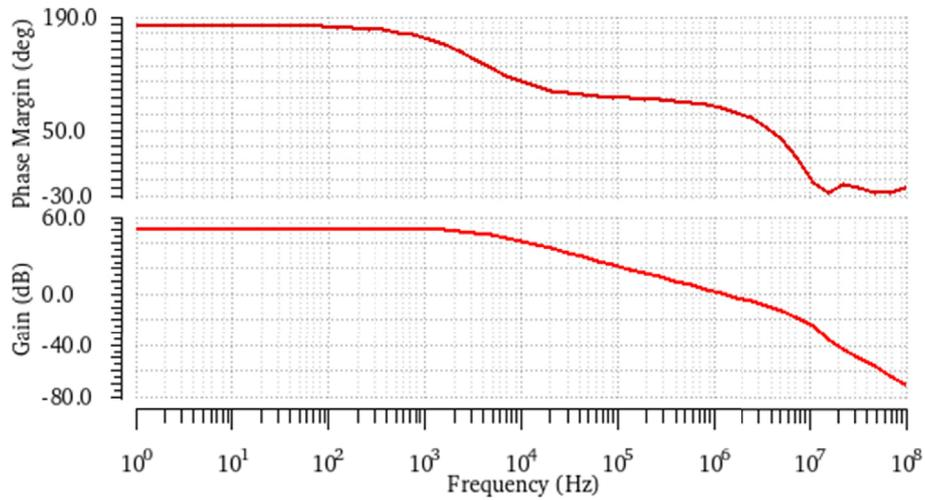
Fig. 7. Phase and gain of the proposed operational amplifier OA1.
