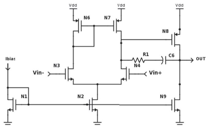
Fig. 3. The two-stages operational amplifier (OA2) used in the regulated cascode current source.
