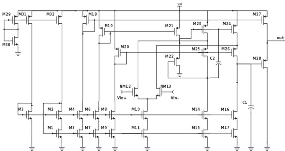
Fig. 2. The proposed 1 V, modified folded cascode operational amplifier with an output buffer stage (OA1).
