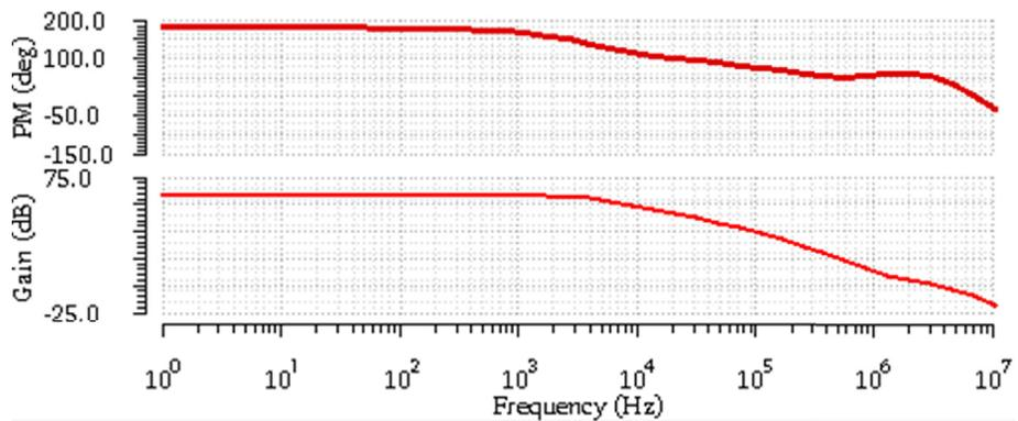
Fig. 8. Phase and gain of the bandgap's main loop formed by OA1 and MP4 loaded with  $(R_1 + r_e)/R_2$ .
