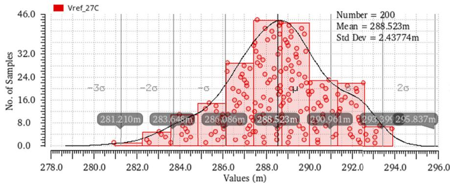
Fig. 13. Monte Carlo simulation results at 27 °C at the supply voltage of 0.9 V.
