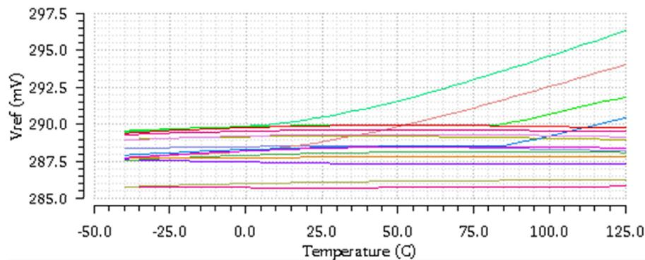
Fig. 5. Output voltage over 32 process corners with 1 V supply voltage varying by  $\pm 10\%$  and temperature ranging within the entire industrial range from  $-40^{\circ}\text{C}$  to  $125^{\circ}\text{C}$ .
