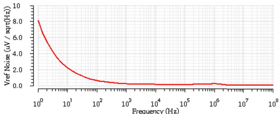
Fig. 6. Noise of the output reference voltage in  $\mu\text{V (RMS)} / \sqrt{\text{Hz}}$ , for 1 V supply voltage and at room temperature.
