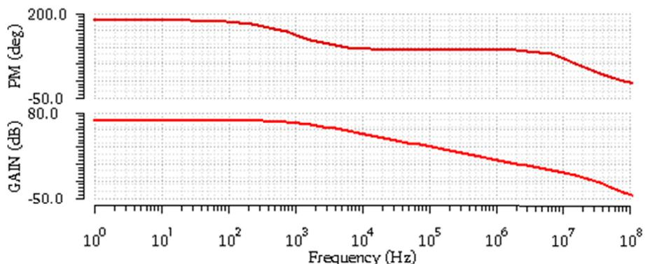
Fig. 9. Phase and gain of the bandgap's second loop, formed by OA2 and MP6 loaded with  $R_4/C_4$ .
