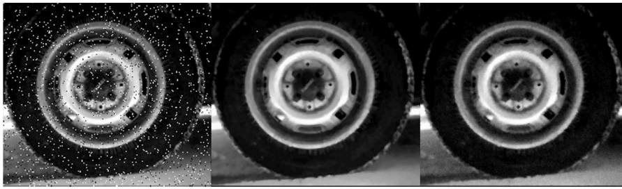
Fig. 11. Denoising using a 3 \times 3 median filter. From left to right: (I) MATLAB's 8-bit noisy image with salt & pepper noise density 0.05, (II) MATLAB's median filtered image, (III) Proposed stochastic median filter with sequence length N = 256 and register size m = 3 -bits.
