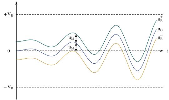
FIGURE 1. Proposed power stage’s continuously tracking rails.
