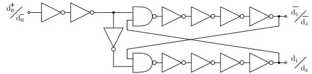
FIGURE 8. Non-overlapping clock generator.
