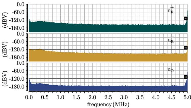
FIGURE 13. Class-CTA rails and output DFTs for an 1 kHz, 1 V input.
