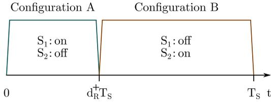
**FIGURE 4.** Positive-rail buck-converter configurations and timing.
