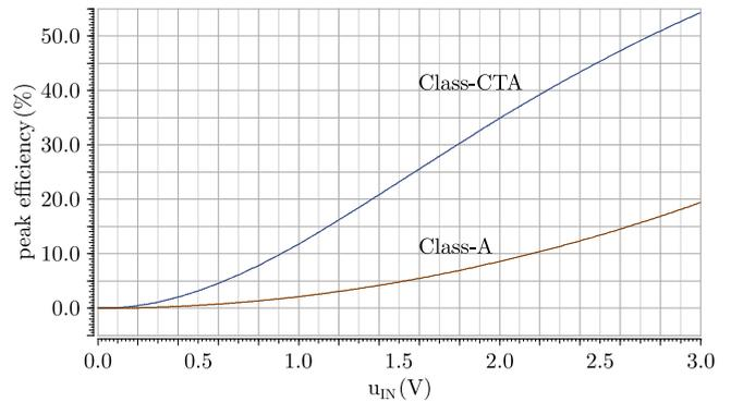
FIGURE 19. Class-CTA vs. Class-A power stage efficiency.
