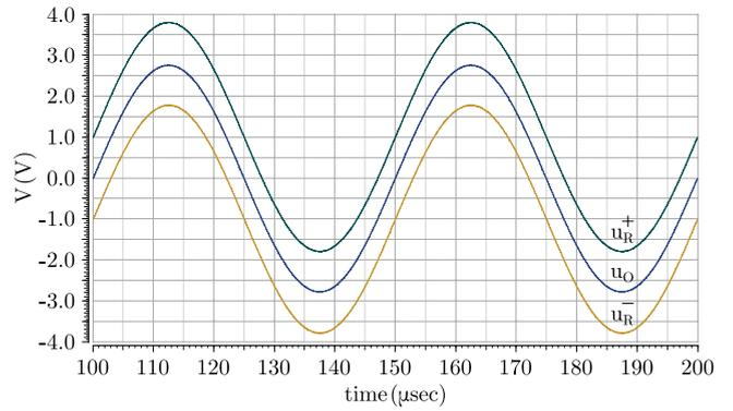
FIGURE 14. Class-CTA rails and output for a 20 kHz, 3 V input.
