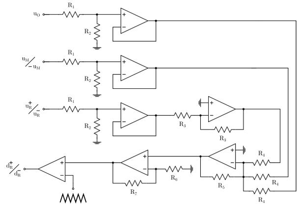
FIGURE 9. PWM control block.
