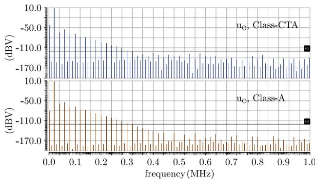
FIGURE 18. Class-CTA vs. Class-A output DFTs for a 20 kHz, 3 V input.
