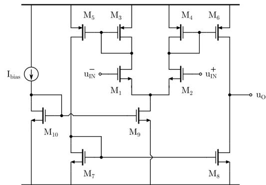
FIGURE 10. Operational amplifier used in the PWM control block.
