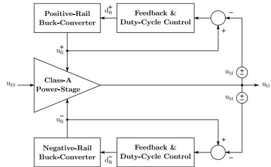
FIGURE 2. Proposed power stage’s system–level architecture.
