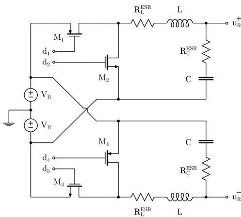
FIGURE 7. Positive- and negative-rail buck-converters of Class-CTA.
