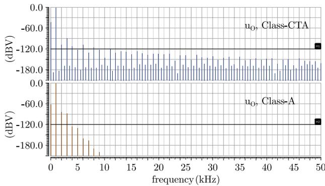
FIGURE 17. Class-CTA vs. Class-A output DFTs for an 1 kHz, 1 V input.
