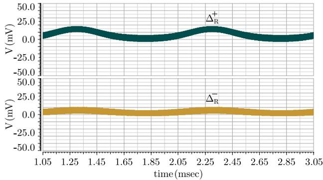
FIGURE 12. Class-CTA rails' error for an 1 kHz, 1 V input.
