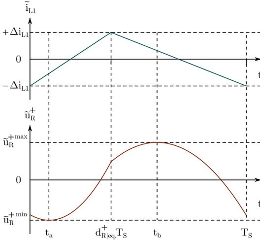
**FIGURE 5.** Positive-rail buck-converter's inductor current ripple and output voltage ripple waveforms.
