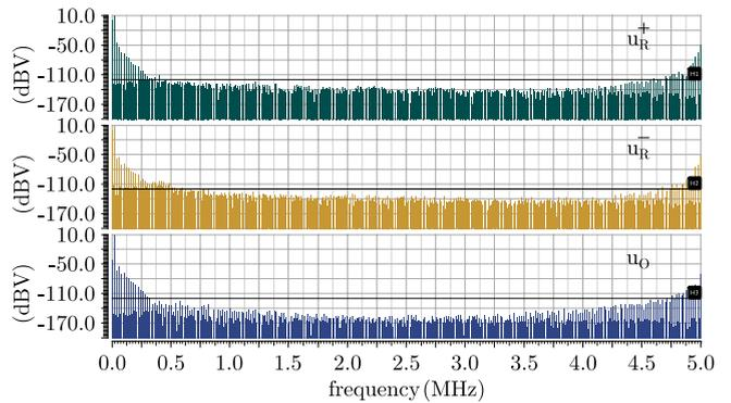
FIGURE 16. Class-CTA rails and output DFTs for a 20 kHz, 3 V input.
