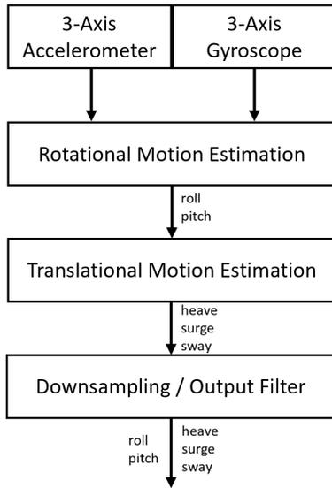
Fig. 2: Data processing flow of the proposed IMU.
