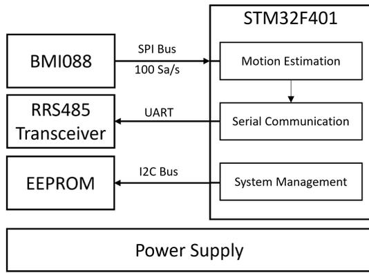
Fig. 1: Top-level system architecture of the proposed IMU.
