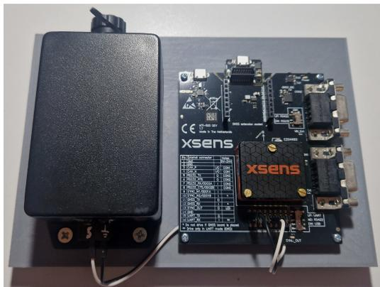
Fig. 4: Designed IMU along with reference IMU (Xsens MTi-630) mounted on a rigid board.
