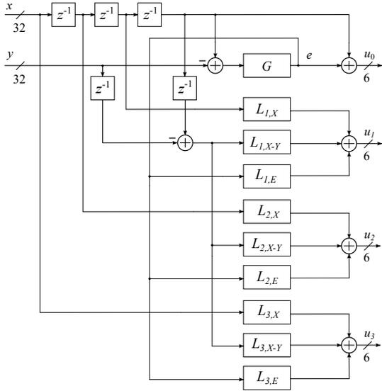
Fig. 1. The designed MSLA SDM loop filter architecture.
