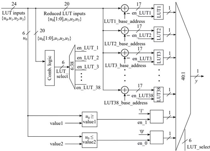
Fig. 2. The designed MSLA SDM LUT architecture.
