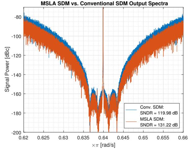
Fig. 3. MSLA SDM vs. conventional single-bit SDM output power spectra.
