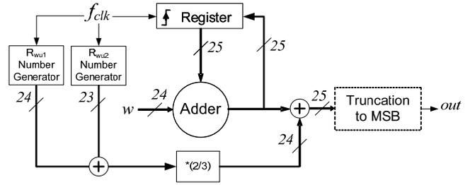
Figure 15. Block diagram of a phase dithered PDDS core of 25-bit, using Approximation II for random sequence generation. (FPGA implemented)
