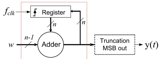
Figure 2. Pulse Direct Digital Synthesizer (PDDS) core.
