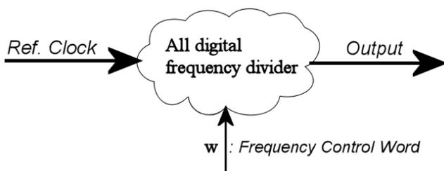
Figure 1. Typical DADFS functionality diagram.
