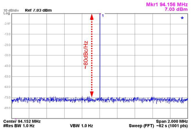
Figure 16. FPGA Implementation (spectrum analyzer measurement)
