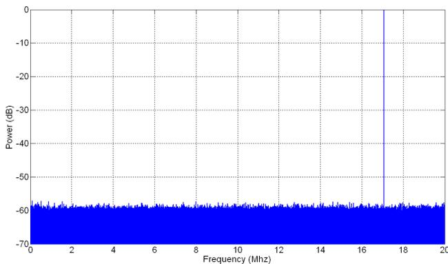
Figure 9. Spectrum of a phase dithered PDDS using the proposed (optimal) dithering sequence (Matlab,  $f_{clk} = 40$  Mhz).
