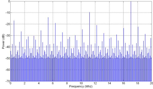
Figure 3. Output spectrum of PDDS (Matlab,  $f_{clk} = 40\text{MHz}$ ).
