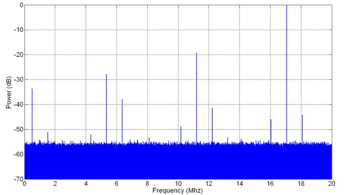
Figure 6. Spectrum of a phase dithered PDDS using a white and uniform noise source (Matlab,  $f_{clk} = 40\text{MHz}$ ).
