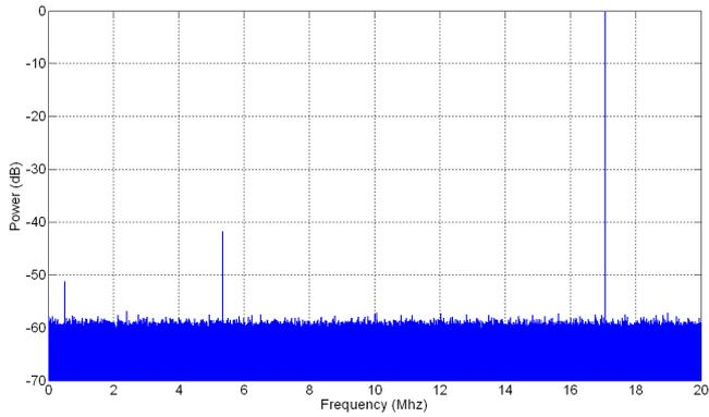
Figure 13. Spectrum of a phase dithered PDDS using Approximation-II type sequence (Matlab,  $f_{clk} = 40\text{MHz}$ ).
