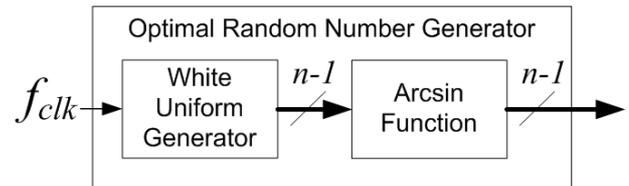
Figure 10. Method for generating the optimal sequence.
