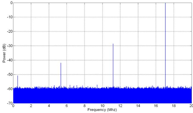
Figure 12. Spectrum of a phase dithered PDDS using Approximation-I type sequence (Matlab,  $f_{clk} = 40\text{MHz}$ ).
