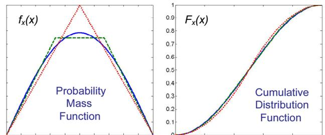
Figure 11. Probability Mass Function and Cumulative Distribution Function of: an ideal sequence (blue solid), approximation I (red dotted, of Triangular form) and approximation II (green dashed, of Trapezoidal form).
