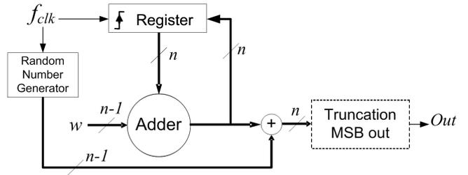
Figure 5. Phase dithered PDDS core.
