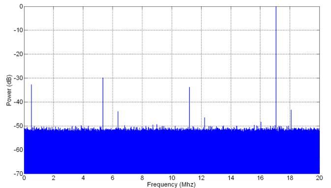
Figure 7. Spectrum of a phase dithered PDDS using a white and uniform noise source of increased strength (Matlab,  $f_{clk} = 40\text{MHz}$ ).
