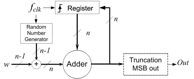
Figure 4. Frequency dithered PDDS core.
