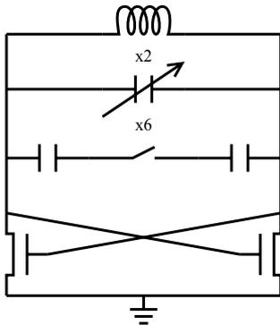
Figure 5. The core circuit of the VCO
