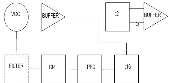
Figure 4: Architecture of the IF PLL
