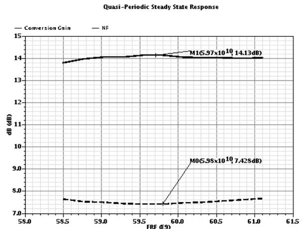
Figure 7. Noise figure and Conversion Gain of the RFFE
