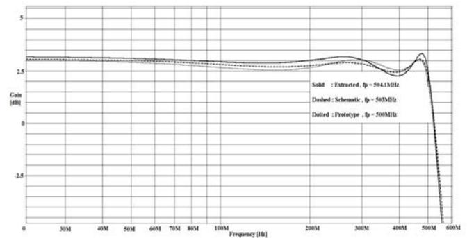
Figure 8: Frequency response of the filter
