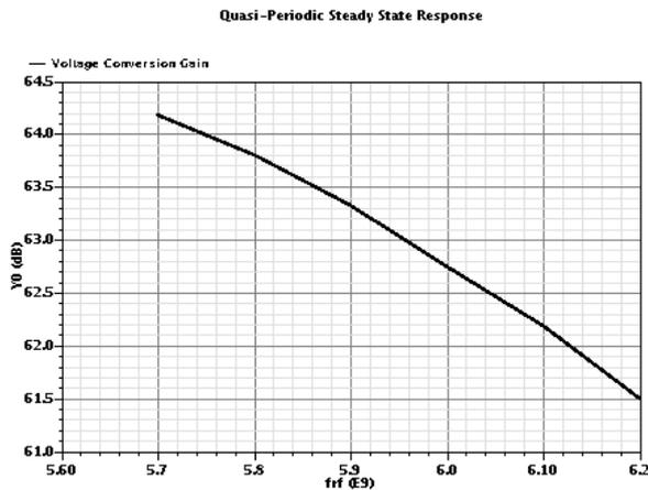
Figure 9. IF and Baseband Voltage Conversion Gain
