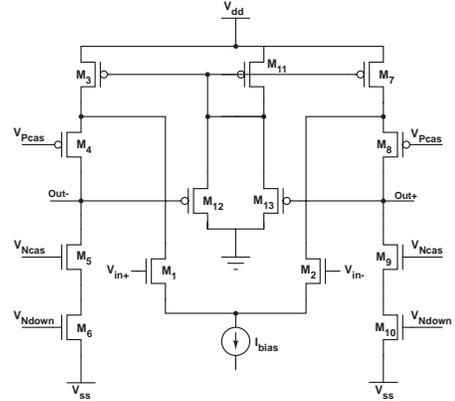
Figure 7: The transconductor’s circuit
