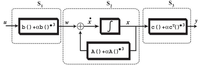
Figure 3: Block diagram of the weakly nonlinear  $G_m - C$  filter
