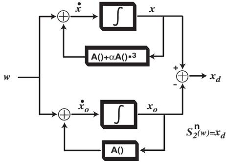
Figure 4: Definition of operator  $S_2^n$
