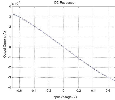
Fig. 5. I-V characteristic of the transconductor in Fig. 4.
