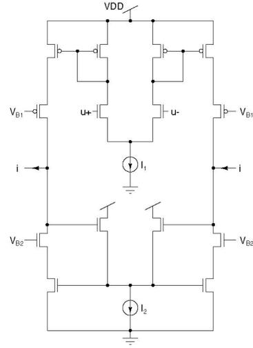
Fig. 4. Schematic of the transconductor used in Cadence simulation.
