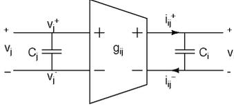
Fig. 2. Fully differential  $G_m - C$  block.
