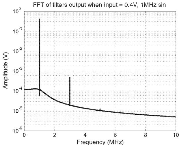
Fig. 7. Fast Fourier transform of the low-pass filter output in Figure 3 driven by input signal  $u(t) = 0.4V \sin(2\pi \cdot 10^6 t)$ .
