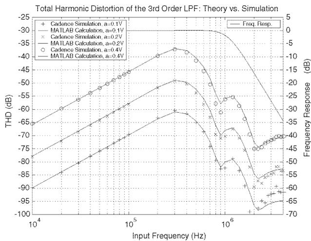
Fig. 6. Simulation results of the low-pass filter shown in Figure 3. The top solid line is the frequency response. The three lower solid lines are the distortions of the filter when driven by 0.1V, 0.2V and 0.4V input signal. “o”, “x” and “+” correspond to SPICE (CADENCE) measurements.
